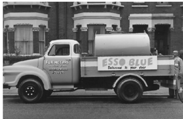
1957-This truck (equipped with a metering device and ticket printer) was used to deliver Esso Blue kerosene to householders in London.
